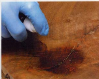
Spray cyanoacrylate accelerant into the gap. This prepares the check for a fast-drying repair.
