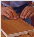
Tools for trimming. Use a block plane to trim most of the excess edging flush to the plywood surface (left). Angle the sole of the plane to achieve a cleaner cut. A cabinet scraper finishes the job (above).
