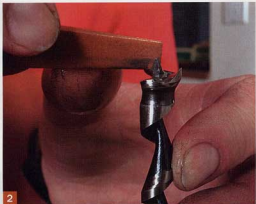
1 Start with the wing. A few short strokes with a fine-grit auger-bit stone sharpens the wing of the bit.
