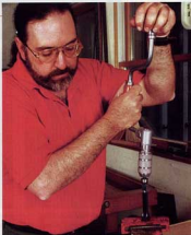
Interchangeable pilots. The reamer comes with an assortment of pilots to fit various sizes of chisels.
