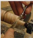
The tenon is cut first. Make a series of cuts with the V-parting tool using a wrench as a guide.
