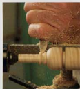
Cut a small cove. Center the spindle gouge and gradually raise the handle to increase the depth.
