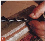
5 Hone the flutes. The flutes of the bit can be smoothed by rotating the bit counterclockwise on a flat stone.
