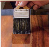
Prevent pooling. With thicker finishes, leave a gap between strokes.
