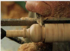
Worry-free beads. With the depth of the bead already defined on both sides by the V-parting tool, round over the sides of the bead with a series of light cuts.
