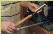
Roughing-out gouge. Rest the handle in a pocket holder and rotate the tool against the grinding wheel.
