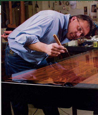
Look out for puddles. Occasionally look at your work from a low angle to check that the finish is being applied evenly. Slow-drying finishes can be leveled simply by rebrushing.
