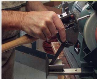
Roughing-out gouge. Rest the handle in a pocket holder and rotate the tool against the grinding wheel.
