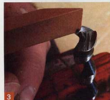
3 On the edge. When sharpening the cutting edge, pull the stone in one direction, working from the leading edge to the trailing edge.
