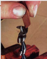
1 Start with the wing. A few short strokes with a fine-grit auger-bit stone sharpens the wing of the bit.
