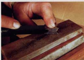
Remove the bevel burr. Use a fine-grit flat stone to remove the burr on all four sides of the chisel.
