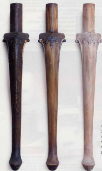
From dark to light. By using a stripper, a darkly stained piece (left) can be lightened (center). If an even lighter tone is desired, the piece may be bleached (right).
