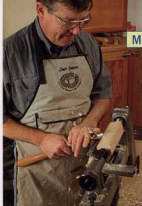
Rounding the billet. Take light passes with the roughing-out gouge to gradually turn the blank round.
