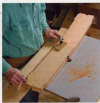
Route the curve one half at a time. Only a half template is needed. Use a bearing-guided bit and work downhill, with the grain. Then flip the workpiece and reattach the template.
