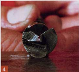
4 Hone the tip. Rotate the tip of the bit clockwise on the flat stone to hone the outside surfaces. Use a light touch here.
