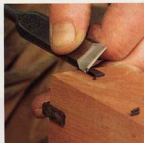
Soften the edges with a chisel. After gluing the ebony splines into place, pare and sand them to a gentle curve.
