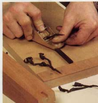
Plane the ebony stock to fit. Get it close on the tablesaw, then use a block plane to creep up on a tight fit.
