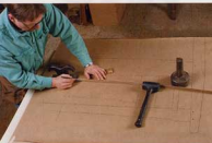
Design the curves using a flexible batten. Rogowski lays out the curves on full-sized drawings of the footboard and the headboard. Only half of each symmetrical view is necessary.
